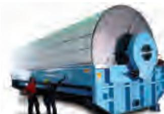
Rotary Vacuum Drum Filter
